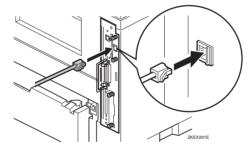
Connect the other end of the network interface cable to the network.
