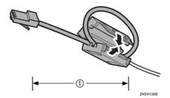
Attach the network interface cable to the jack on the board.
