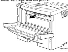
While lifting the front side of the toner cartridge, pull it out of the printer.
