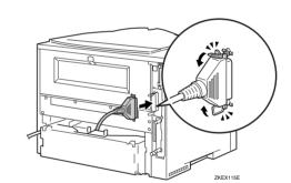
Attach the other end of the interface cable to the interface connector of the computer. Secure the cable.
