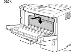
Close the front cover by pressing the indentations on the left and right sides.
