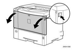
Remove the fixing material inserted between toner cartridge and the printer.
