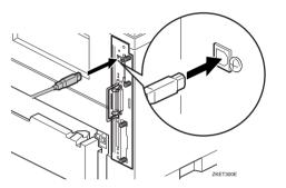
Attach the other end of the interface cable to the USB interface connector of the computer or the USB Hub. Secure the cable.
